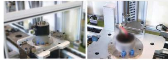
粉塵清潔 Dust cleaning the stator and the internal body 置入波形墊圈 Place in wave washer
