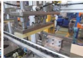
檢測三相電壓端子 Testing three-phase voltage terminal
