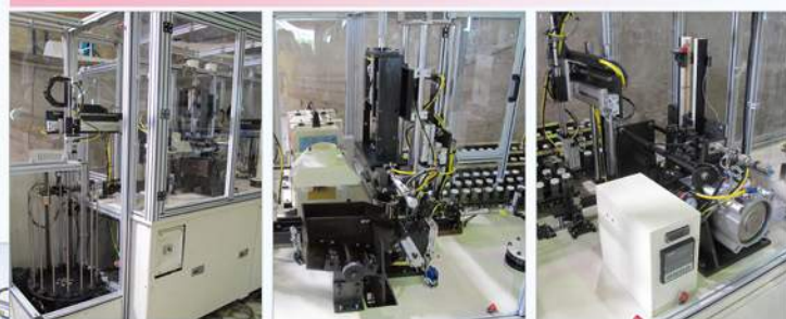
◆供料台 Feed Table ◆軸心熱合 Heating and Inserting ◆脫拔力 Pull-off Force tester
