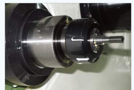
擠光刀具0.6S 0.6S Burnishing tool
