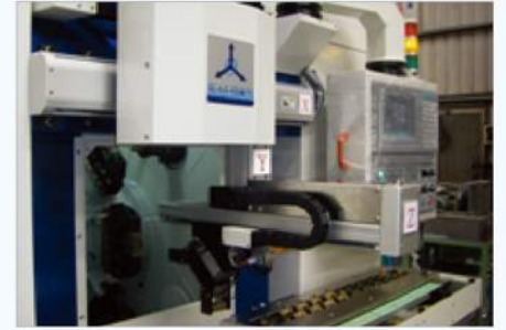
位移伺服機械手搭配簡易送料成本低 Servo-controlled robotic arm works with basic feeder to lower cost.
