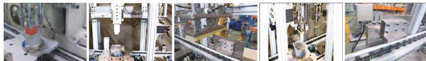
自動螺絲站 Automatic screw tightening station 檢測軸向間隙長度 Testing axial clearance length 檢測三相電壓端子 Testing three-phase voltage terminal 檢測扭力值 Inspect screw tighten torque 使用條碼分辨料號 Using the bar code to distinguish workpiece
